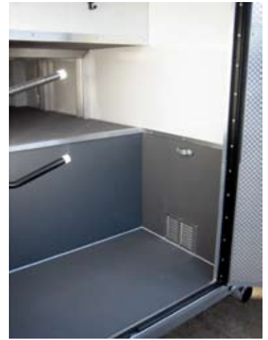
Grey Multifloor used to line the locker of this impressive horsebox and also used for the van floor below
